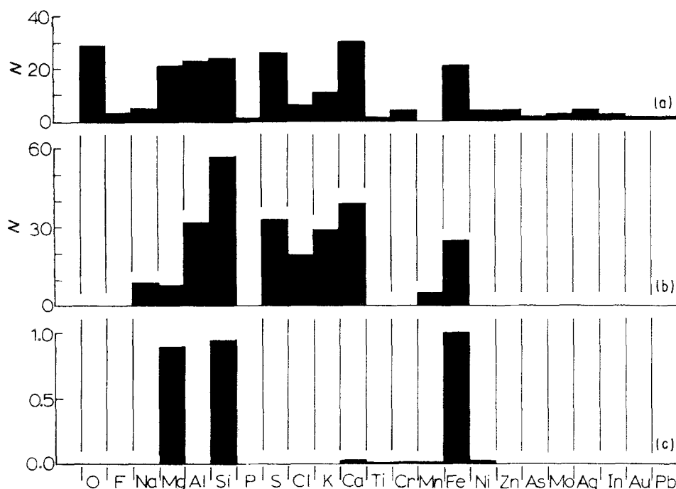
Figure 3 Comparisons of elemental frequencies or distributions in particulate regimes. (a) Experimental analysis of approximately 100 particles or debris fragments extracted from a small area in D09 from LDEF (Fig. 2); elemental frequency of occurrence is denoted by N . (b) Elemental analysis of more than 100 particulates in the upper atmosphere (3 km) over central New Mexico, USA, and regarded as ice-forming nuclei (IFN); elemental frequency of occurrence is denoted by N as in (a). (c) Elemental abundance (normalized with respect to iron) or proportion averages for chondritic micrometeoroid particles or interplanetary dust particles (IDPs) after data in [11]. This distribution contains small amounts of nickel, chromium and titanium as shown.
